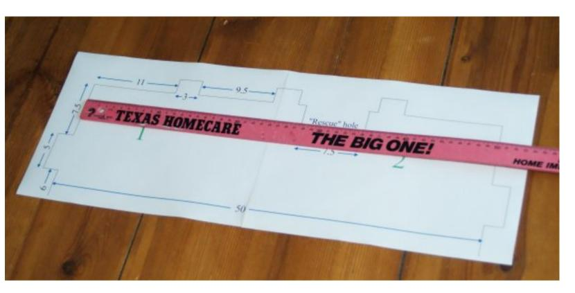
Add sheets 3 and 4 in a similar way, checking this time that as well as maintaining the 50 cm width, the 6 cm gap between side tabs is exact. Ensuring sheets 1 and 2 have not shifted, tape at the joins as before. Continue down the sheets, checking and taping as you go. You may want to add extra tape on the back to ensure the whole plan can be picked up without falling apart.
