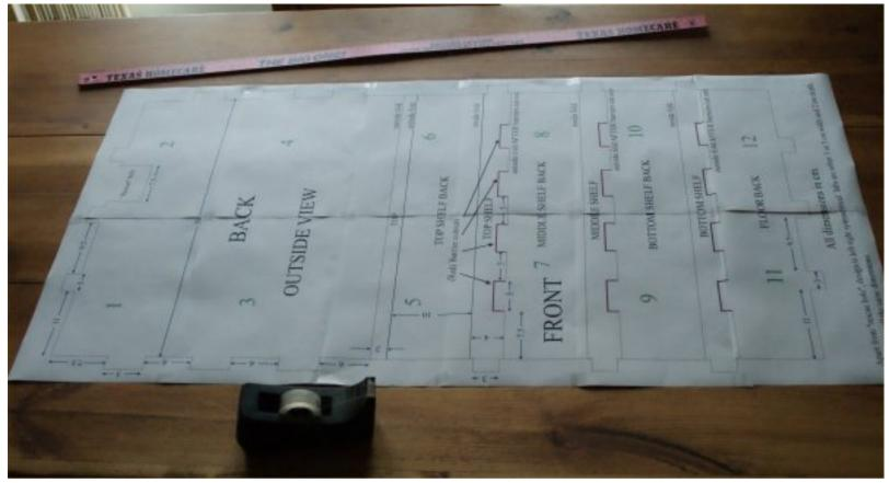
When the full plan is complete, lay it on the cardboard, ensuring existing folds are positioned correctly i.e. not under tabs or the barrier cutouts and only if possible where folds are needed. Attach the plans to the cardboard with a few pieces of tape. Place plans and cardboard over a flat surface already covered in something thick to protect it – old copies of Radio Times are ideal!
