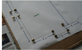
"Join the dots", using felt pen rather than biro so as not to damage the cardboard. It's probably easier later if you use continuous lines for cuts (1st photo), along with dashed lines on the front of the card for inside folds (2nd photo) and on the back for outside (3rd photo).
