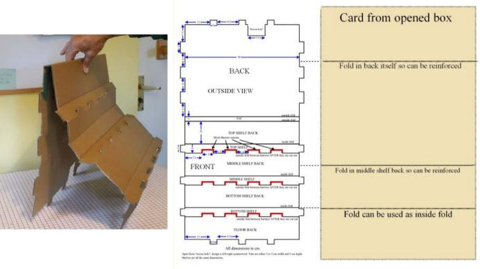
Strategy A: If you intend to draw out the plans directly on to the cardboard, do so now. Note where fold lines are to be on the visible (outside) face i.e. "inside folds" and where on the invisible face i.e. "outside folds". Don't draw fold lines below the barriers, only in between them. It's probably easier later if you use continuous lines for cuts and dashed for folds.
