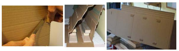
Next, fold the sides up, insert the tabs, score, fold and glue as before. Place the unit on one side on the polythene, lay polythene on top (i.e. on the other side) and add wood and weights sufficient to compress the tabs, though not to threaten to collapse the whole structure! Allow to dry as before.
