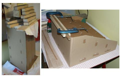
Block off the ends of the support with e.g. small squares of cardboard or filler, to finish the construction. If you're intending to paint any of it, use primer on the tabs and anywhere else where dried glue might be exposed. Exposed corrugation holes could be pinched closed and glued, or filled with wood filler or even plaster filler, though something slightly flexible will last longer.
